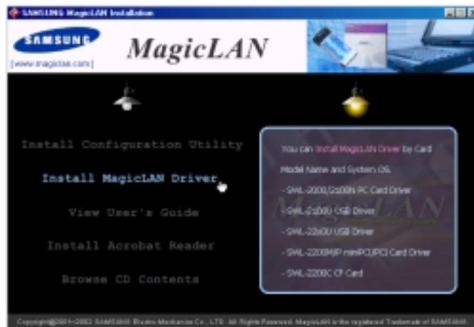
2. You can see the pictures of Wireless LAN Cards by model name.([SWL-2200U Mini USB Adapter](#)). Click on the model name to install it’s driver.
