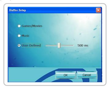
Bigger buffer causes audio transmission delay, but also makes it more stable and reduce the possibility of audio broken due to wireless signal interference.
