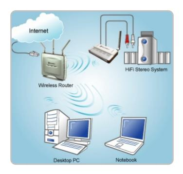
Client or Wireless Client mode allows AW-GA200 device to become a wireless client and connect to another AP. In other words AW-200 now becomes a wireless adapter card to the wireless network to receive wireless audio from PC.
