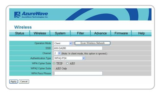
**WPA-PSK (Wi-Fi Protected Access):** The WPA security pre-shared key supports TKIP and AES algorithm. TKIP and AES utilize a stronger encryption method and incorporate Message Integrity Code (MIC) to provide protection against hackers. To use WPA Pre-Shared Key, enter a password in the WPA Shared Key field between 8 and 63 characters long.
