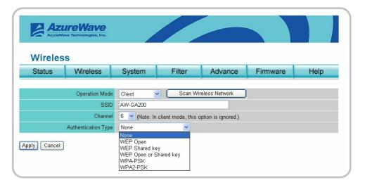
**Wired Equivalent Privacy (WEP):** WEP is a basic encryption method in WI AN.
