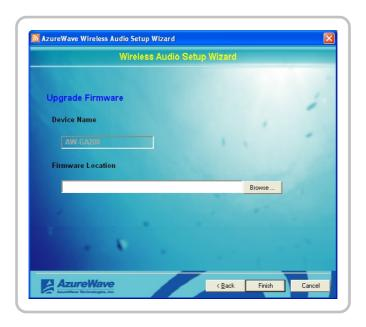
Note: Do not upgrade your firmware through a wireless connection. During upgrade process, please ensure that the power connection and Ethernet connection are not interrupted. Upgrade through wireless connection with power/Ethernet interruption may lead to an irrecoverable damage to the device.
