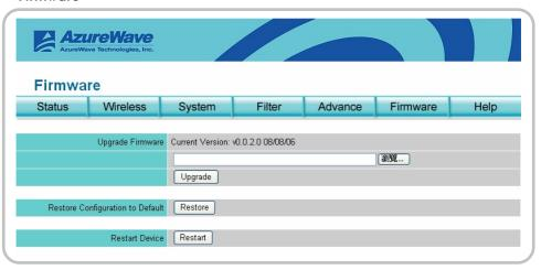
**Upgrade Firmware:** Current Firmware version can be located within the Upgrade Firmware column. In order to start firmware upgrade, you need to download the latest and correct firmware for the device from internet. Click Browser button to locate the firmware file (\*.bin) and then click Upgrade button to upgrade firmware.
