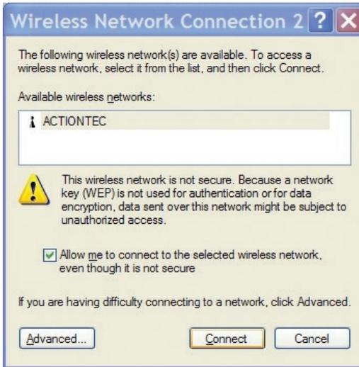
4. Activate the box next to “Allow me to connect to the selected wireless network, even though it is not secure” by clicking in it to cause a check mark to appear.
