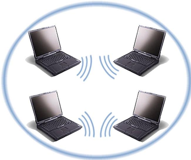
Ad hoc mode is also called peer-to-peer mode or independent basic service set (IBSS). This mode is useful when communicating among many computers locally without the need to connect to printers or file servers on a wired LAN.
