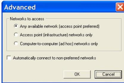
Use this window to select the type of network to which the Adapter connects.
