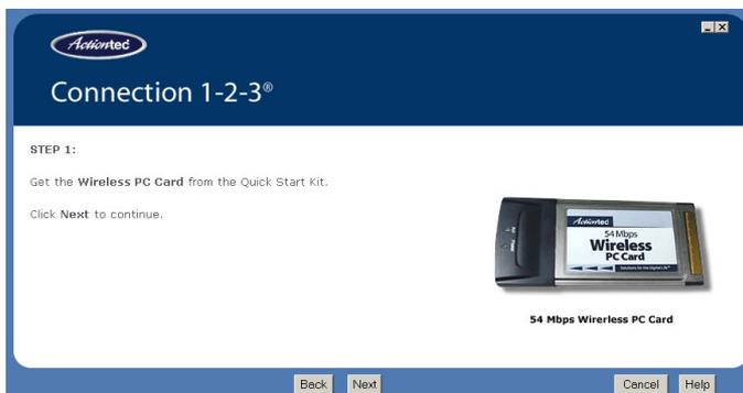
3. Find the PCMCIA (PC Card) slot on the computer. This slot is usually located on the left or right side of the computer. Click **Next**.
